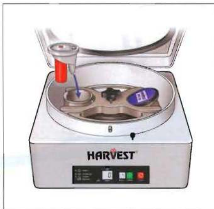
FIGURE 4. Step 5 – Dual chamber disposable is loaded into the centrifuge.
